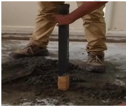
Fig .4 concrete material filling CFST
