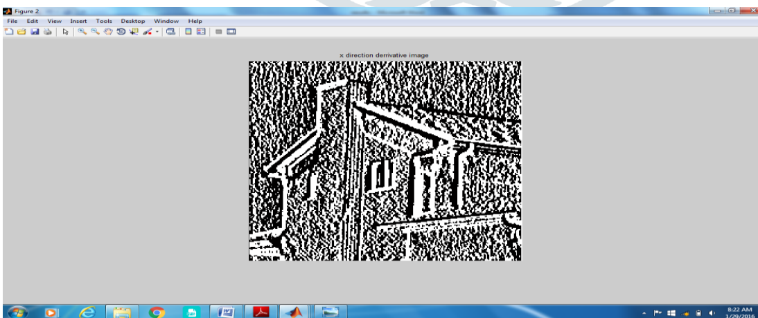
Fig.3 snapshot of horizontal gradient or x-direction derivative image
