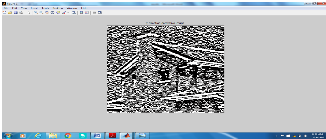
Fig. 4 snapshot of vertical gradient or y-direction derivative image
