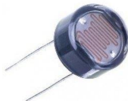
Fig -5: A typical LDR
