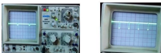
Figure 9-output across TL494 and MOSFET
