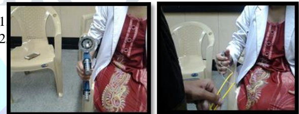
Fig. 5. Photograph of a subject using both FBGHGD and Jammer hydraulic hand dynamometer.
