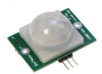
Thus changes of pulses are detected. HT-7133 voltage regulator, BIS0001 micro power PIR motion detector IC, Fresnel lens helps for the operation. When any object is detected the unit will perform some actions to keep them away from the crops. A buzzer may be used in this module to make a noise to keep the unwanted species away.
