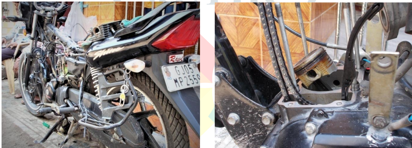
Figure 9: (a) Disassembly of engine of Honda (b) Actual piston
