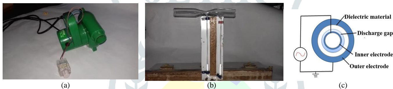
Fig.2: Photograph of (a) air pump which is adjusted by the dimmer to control the air flow rate. (b) The venturimeter which is used to measure the air flow rate. The maximum flow rate that can be measured by this set up is 15.5 l/min. (c) Dielectric barrier discharge
