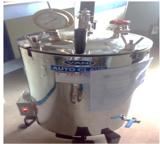
Fig 3.3 sterilizing the solution by using auto-clave equipment
