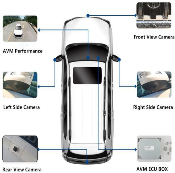
Fig. 3. Bird's eye view camera setup
