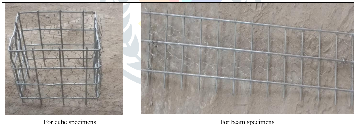
Figure 2: Welded and chicken mesh cages for different specimens
