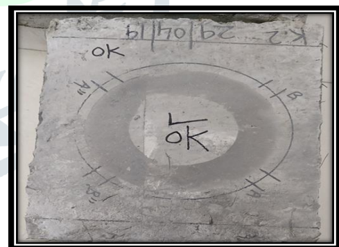
Fig. 2.9 Slab after abrasion test
