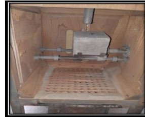
Fig. 2.11 Sample under Sand Blasting
