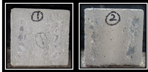
Fig. 2.12 Sample after Sand Blasting
