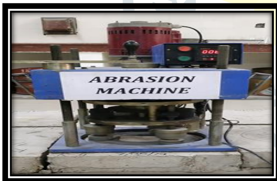
Fig. 2.8 Abrasion resistance test on concrete in slab
