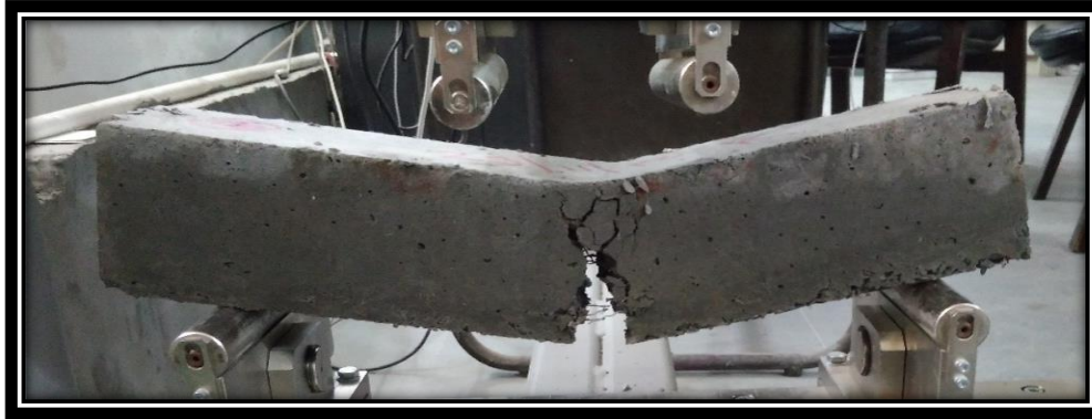
Fig. 2.6 Flexural strength test in progress
