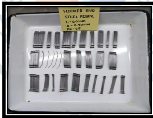
Fig. 2.2 Double Hooked type steel fiber
