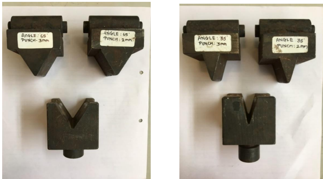
Figure 5 : Punch & die sets with different bend angles available for experimentation
