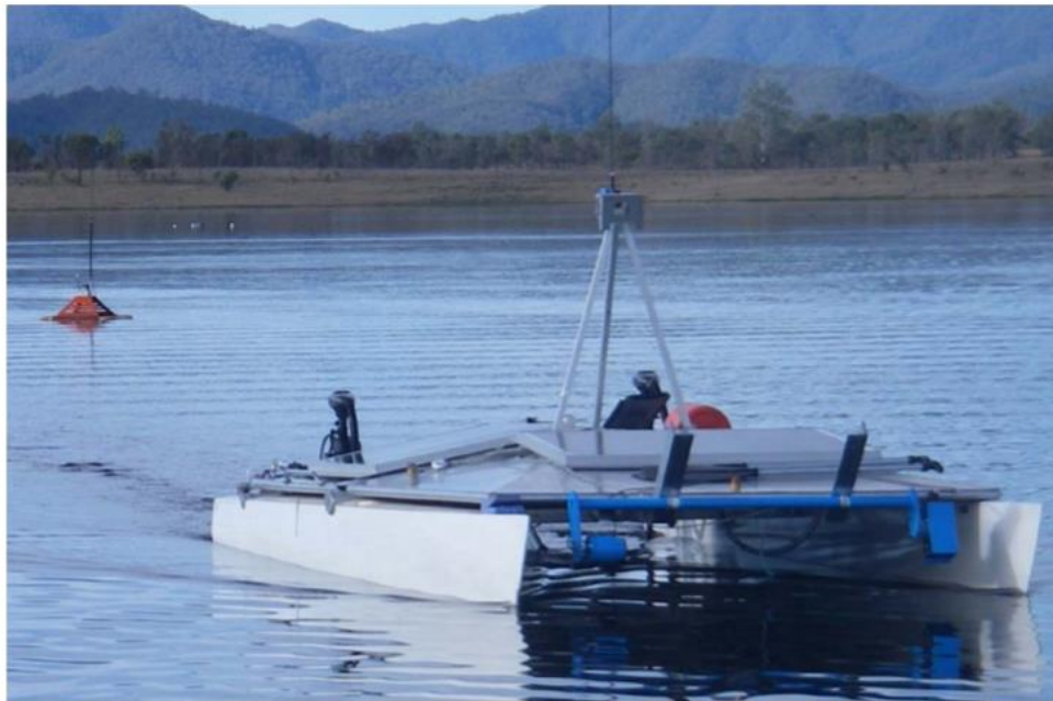
Lake deployment. Robotic boat in the foreground and a floating node in the background.
