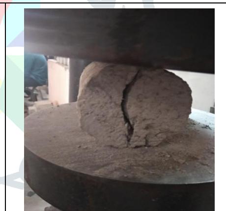
Fig 5.3.2 Split Tensile Failure of GPC
