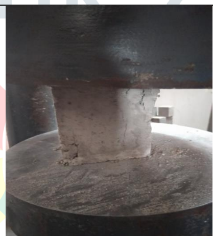
Fig 5.1.2Compression Failure of GPC
