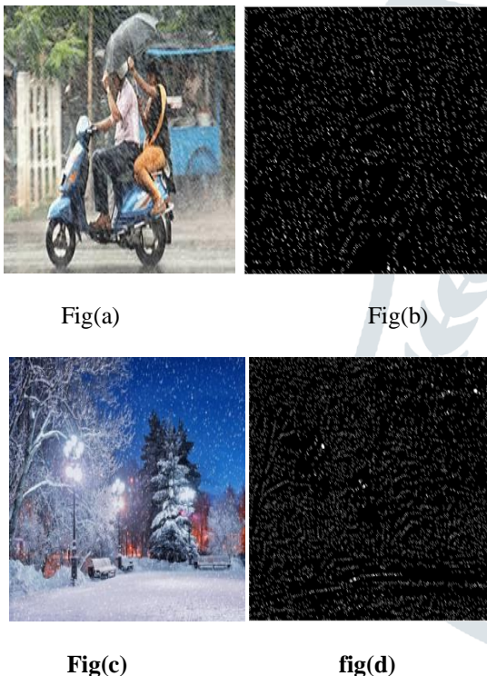
Fig 2: the detection results of rain or snow image (a),(c ) are the input images of rain or snow and (b) and (d) are detection of rain streaks and snowflakes in a image.
