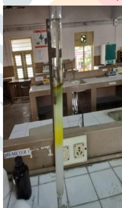
Fig 3. - Isolation of D-limonene form extract of Murraya koenigii by column chromatography
