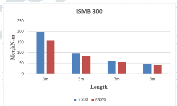
Fig: 7 Length Vs M_{cr} for different spans at ISMB 300
