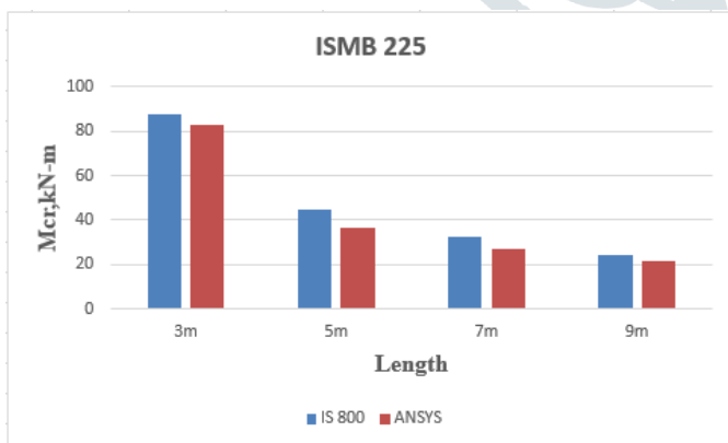
Fig: 6 Length Vs M_{cr} for different spans at ISMB 225
