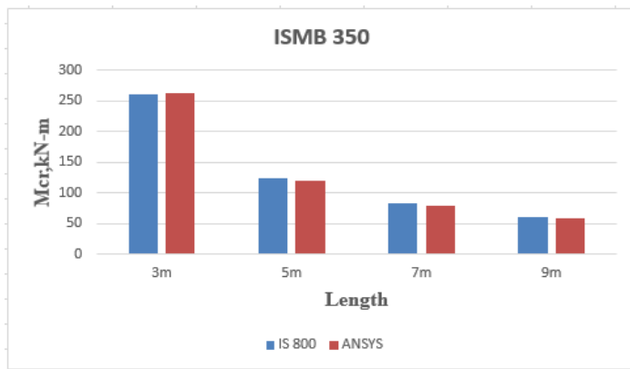
Fig: 8 Length Vs M_{cr} for different spans at ISMB 350
