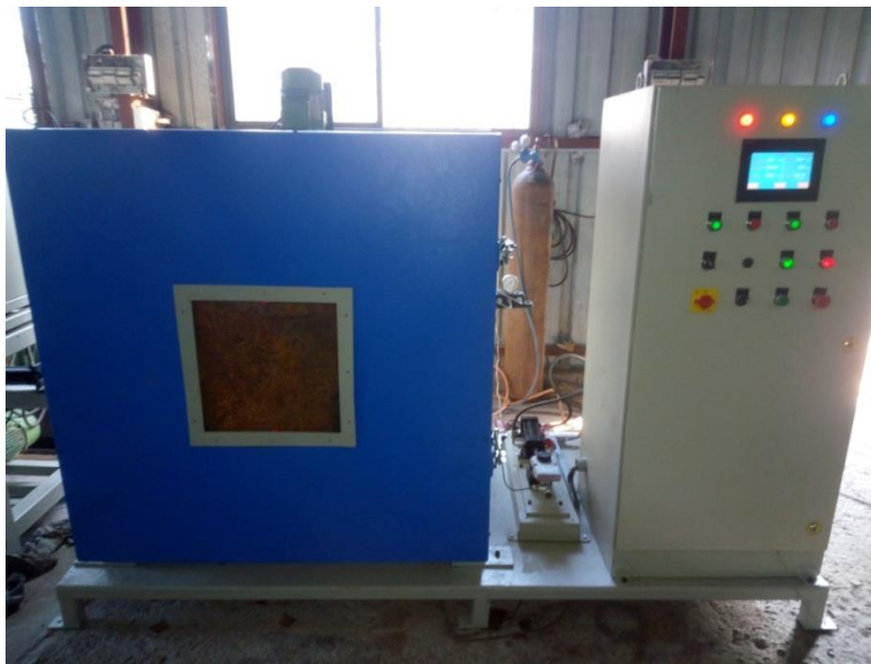
Fig- 7: Hot impulse test setup up (front view)
