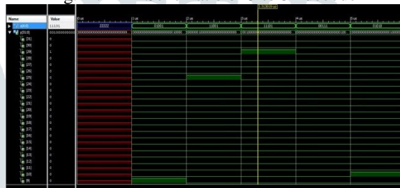
Fig.12. Simulated output of 5 to 32 decoder
