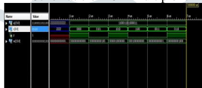
Fig.8.simulated output of 16x1 multiplexer
