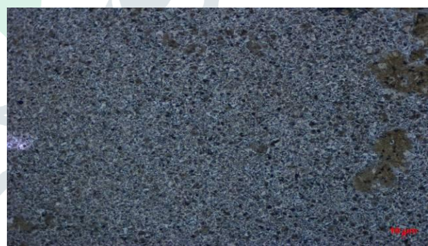
Fig. 6.6. Tempered Sample at 250°C for an Hour at 10X
