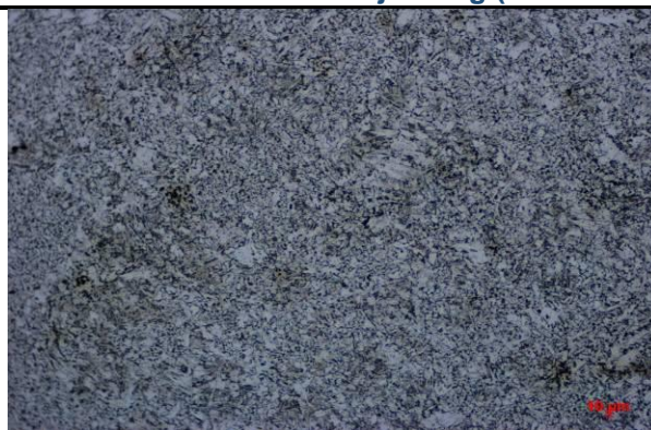
Fig. 6.10. Tempered Sample at 650°C for an Hour at 10X
