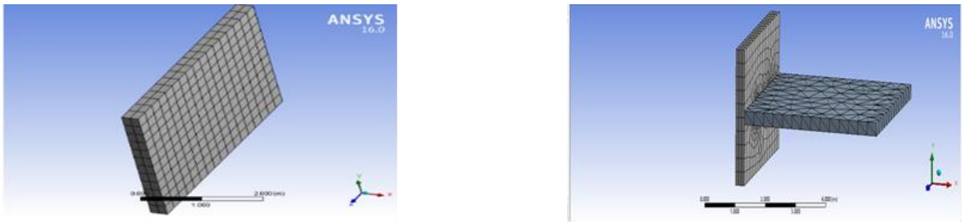
Figure 5 Modelling and meshing of Existing wall and Post-installed wall to slab connection
