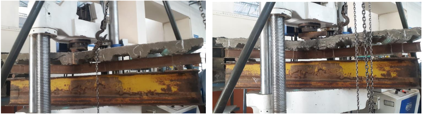
Fig.8 Flexural Testing Process
