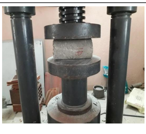
Fig 5.3.2 Split tensile failure of Cylinder
