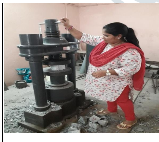
Fig 5.1.1 Compressive test on Cube
