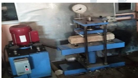
Fig 5.2.1 Flexural test on Beam
