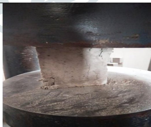
Fig 5.1.2 Compression failure of Cube
