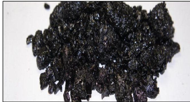
Fig 5: Aggregates after Stripping Test
