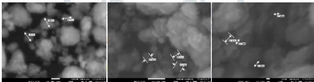
Fig. 2. FESEM images of non-sintered powders after milling time of (a) 2 h, showing particle size 117nm (b) 3 h, showing particle size 39.8nm (c) 4 h, showing particle size 17.7nm
