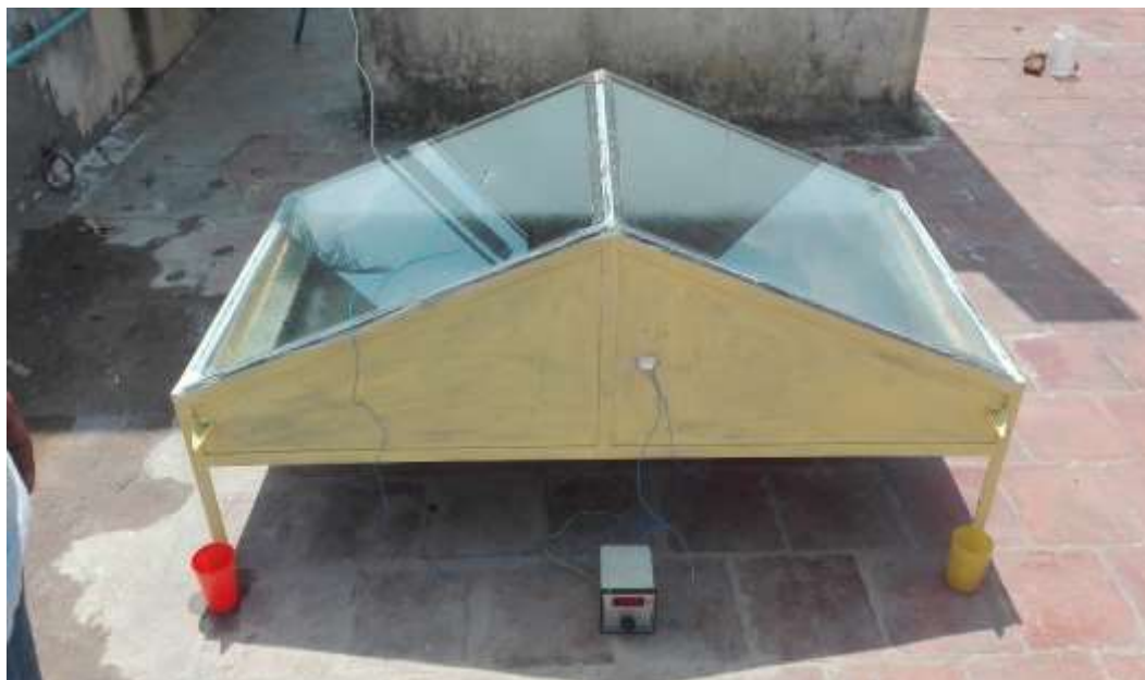
Figure 2 Photographic view of Single Basin Double Slope Solar Still
