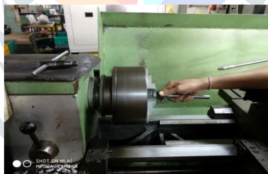
Fig-2: lapping on lathe machine
