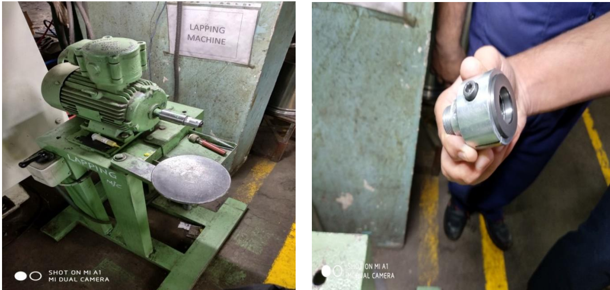
Fig-3 simple lapping machine
