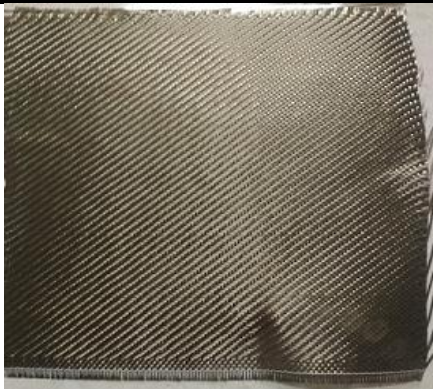
Fig3.1. Basalt Twill Weave Fabric
