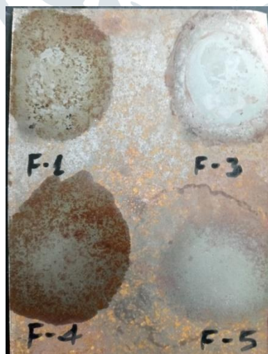
Fig. 4 Metal sheet specimen for comparative results after application of various formulations
