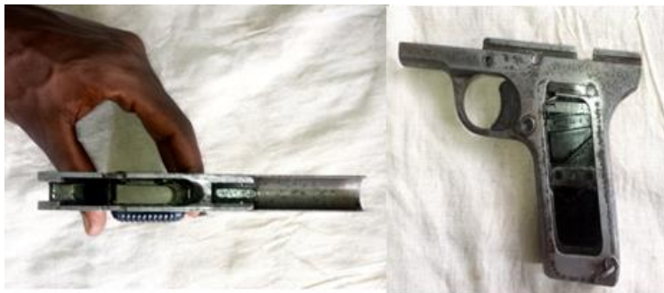
Fig. 6 Part of the same pistol after application of formulation-4
