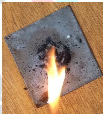
Fig. 7 Carbon ignition test for the removal of carbon
