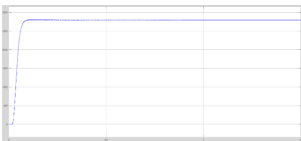
Figure 12. Total power generated by wind turbine
