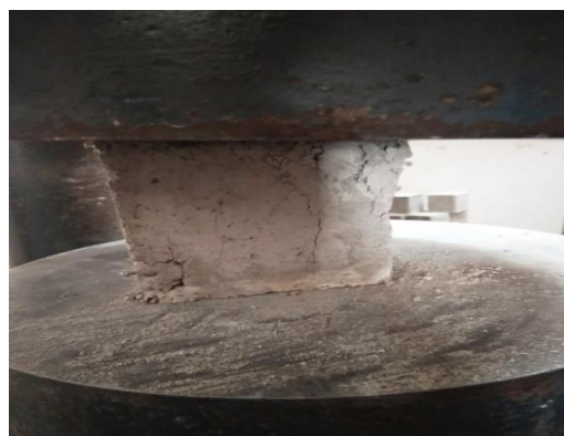
Fig 5.1.2 Compression Failure of GPC
