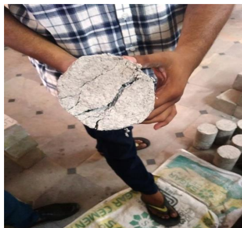
Fig 5.3.2 Split Tensile Failure of GPC
