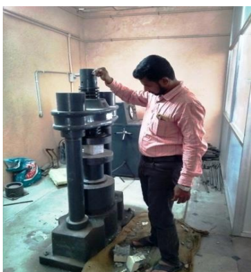
Fig 5.1.1 Compressive test on GPC
