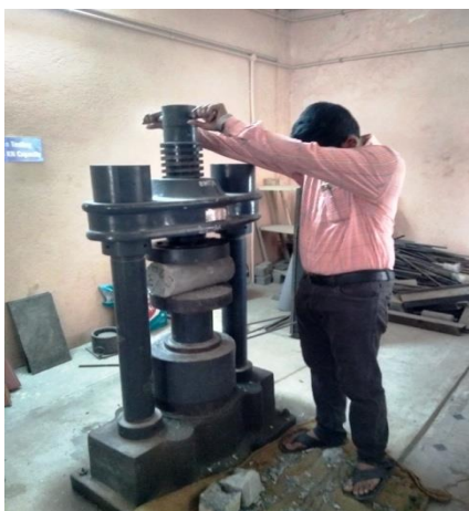
Fig 5.3.1 Split tensile test on GPC
