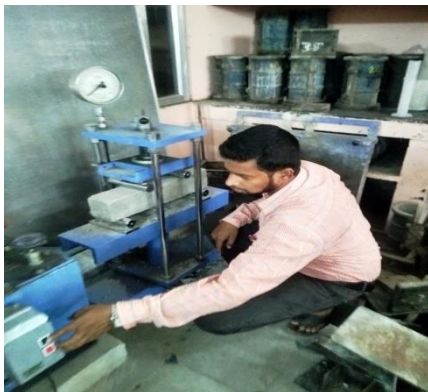
Fig 5.2.1 Flexural test on GPC
