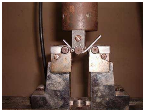
Figure 4.3 Loading arrangement for flexural
