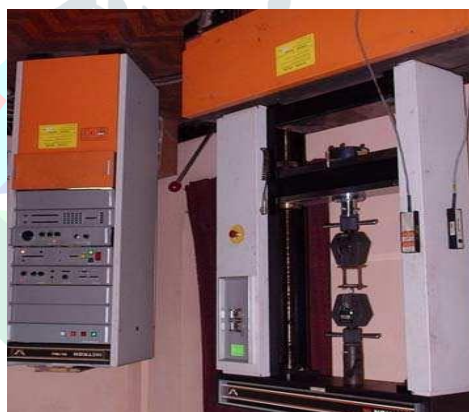
Figure 4.1 Experimental set up for tensile test
