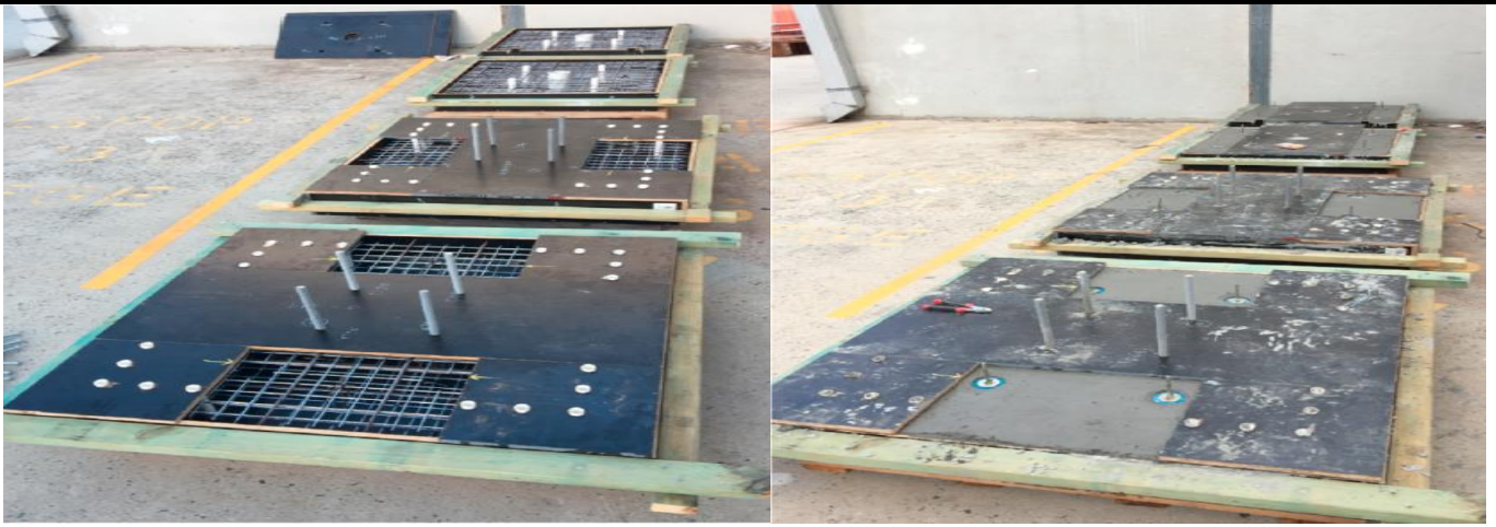
Figure 3.1 table shakers with fastening fixtures.
