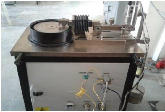
Fig.6 Wear test machine setup and specimen
