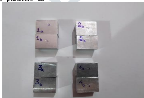
Fig.5 Hardness Test Specimens
