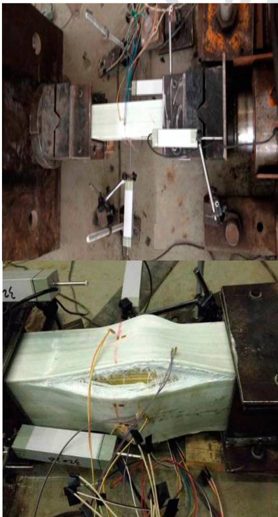
Figure 3.3 Schematic of test specimen with compression testing apparatus.
