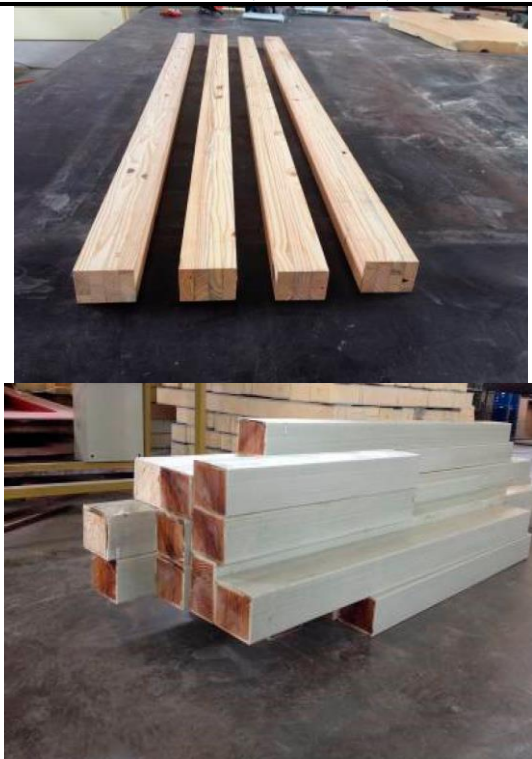
Figure 3.1 Pine wood columns for test specimen
