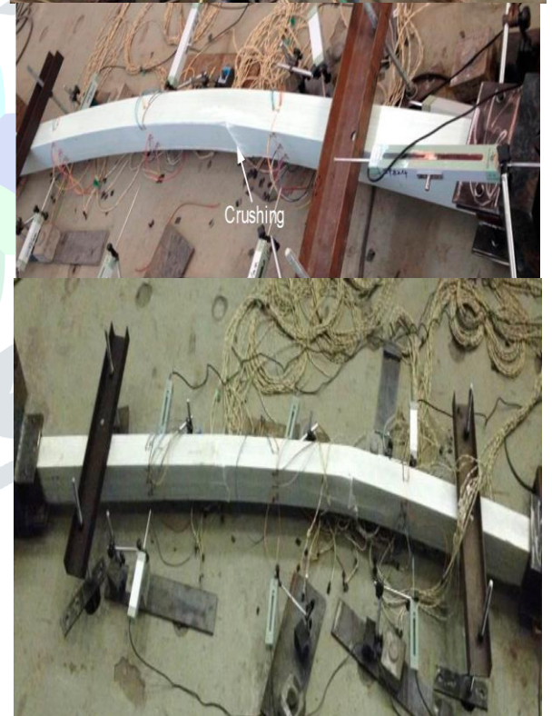
Figure 3.5 Representation of buckling of pine wood coated with epoxy reinforced polymer.
