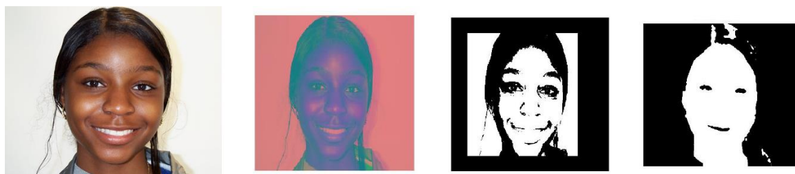
Fig. 2. The skin-color segmentation:(a) Original face image (b) Image in YCbCr space(c) Similarity image (d) Binary image morphological operations
