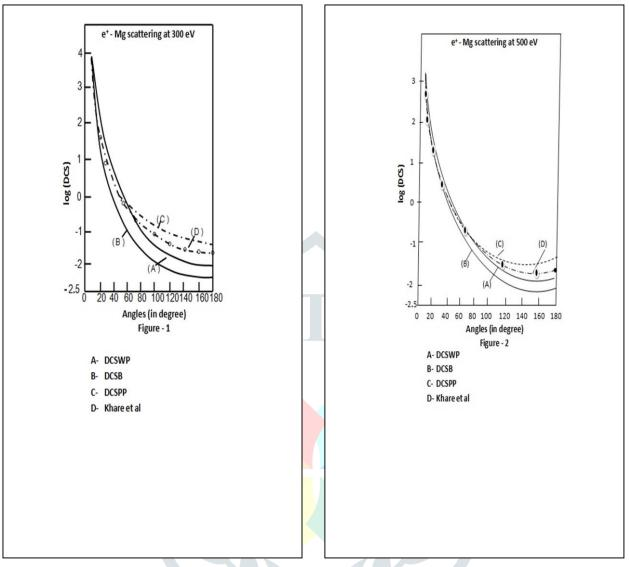
At 300 eV, curve B lies below curve A. With increase of energy, closeness between curve A and B has increased. This is expected result.
