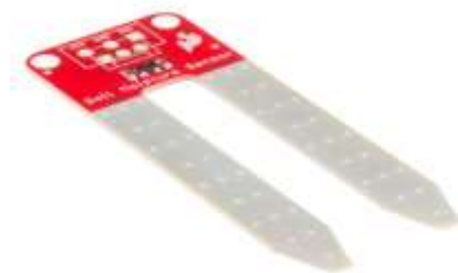
Figure 8: soil moisture sensor UV sensor:
