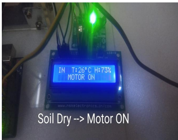
Fig.18: shows motor ON condition when soil dry
