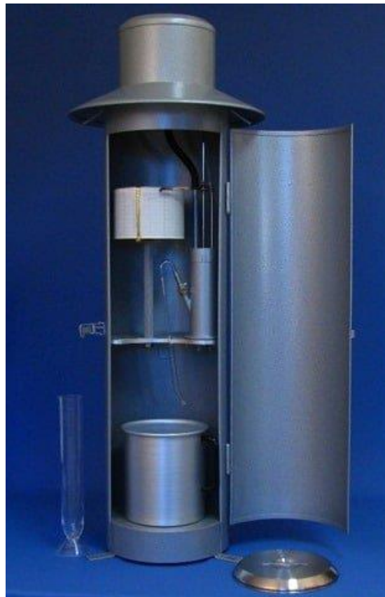
Fig. 5 Natural Siphon or Float Type Rain Gauge
