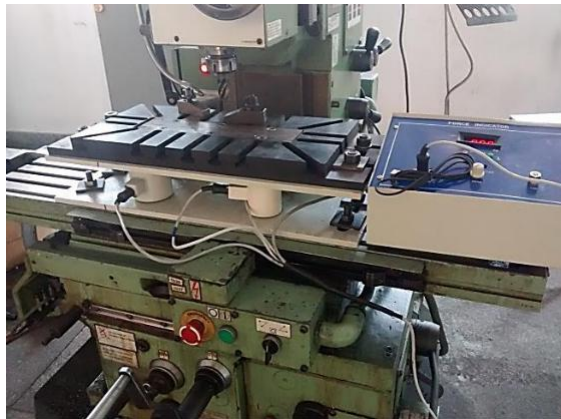
Fig. 2: FSW set up on Universal Milling Machine with vertical head
