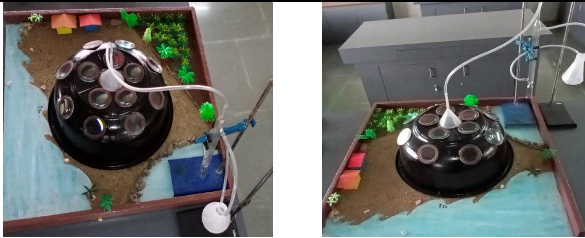
Fig 1 Solar Water heater by using convex lens
