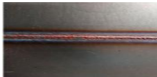
Specimen 2 of ( Ti-6Al-4V) laser welded
