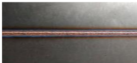
Specimen 1 of ( Ti-6Al-4V) laser welded
