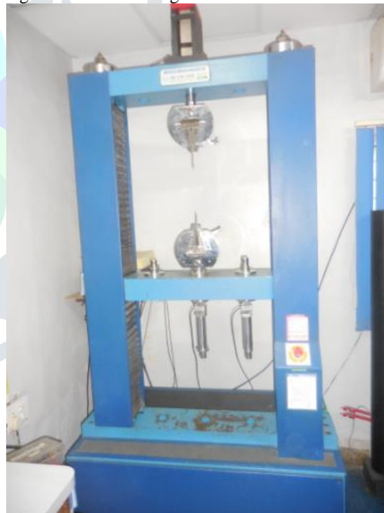
Figure UTM frame
