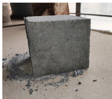
Fig 3.14. Cubes After Compressive Strength Test
