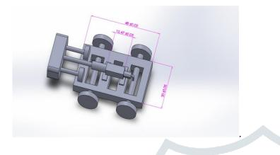
• The length of the robot is 48 cm and the width of the robot is 30 cm. The diameter of the wheels is 7 cm also a belt drive is used over the wheels to increase the friction force so that there will be less amount of deflection in the robot when the piston is in working condition. The bore of the piston is of 2.5 cm and the maximum length of the stroke is of 10 cm.
