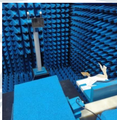
Fig.8. Measurement setup for antenna measurement
