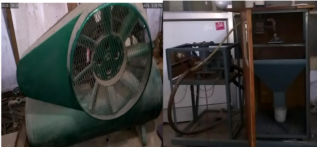
Fig. 1 Experimental setup for Abrasive Jet Drilling Process
