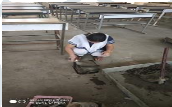
Fig. 3.2 casting of concrete cube
