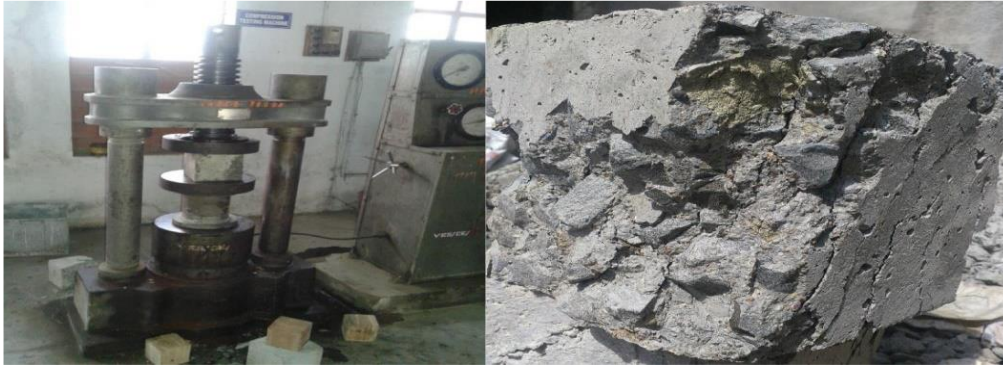
Fig. 4.1 Compressive Test on Concrete
