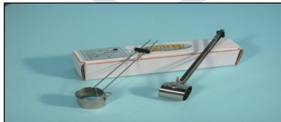
Fig. 3.4 Soundness Test of Cement by le-chatelier apparatus
