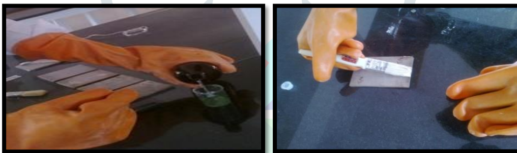
Figure : Preparations and Application of Activated Flux Powder
